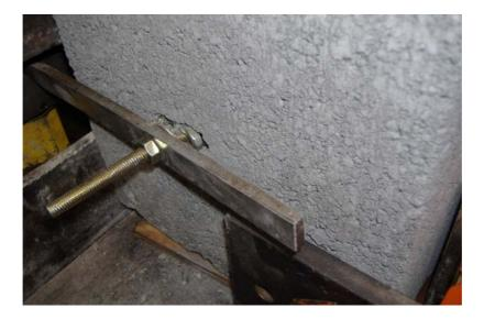
Plate 6 - Failure of Test Specimen in Shear
