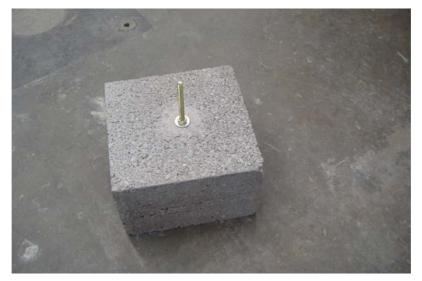
Plate 3 - Showing Test Sample Prior to Tensile Test
