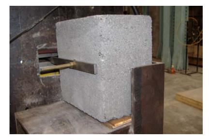
Plate 4 - Shear Test on Test Specimen
