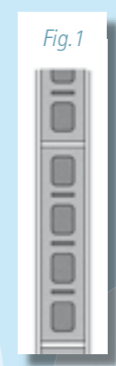
Fig.2 Bescrete Cellular Blocks should be laid vertically, voids down.
