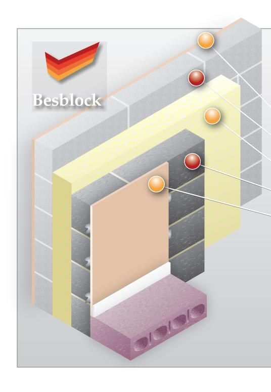
Besblock Medium Density Block Fully Filled Cavity Batt
