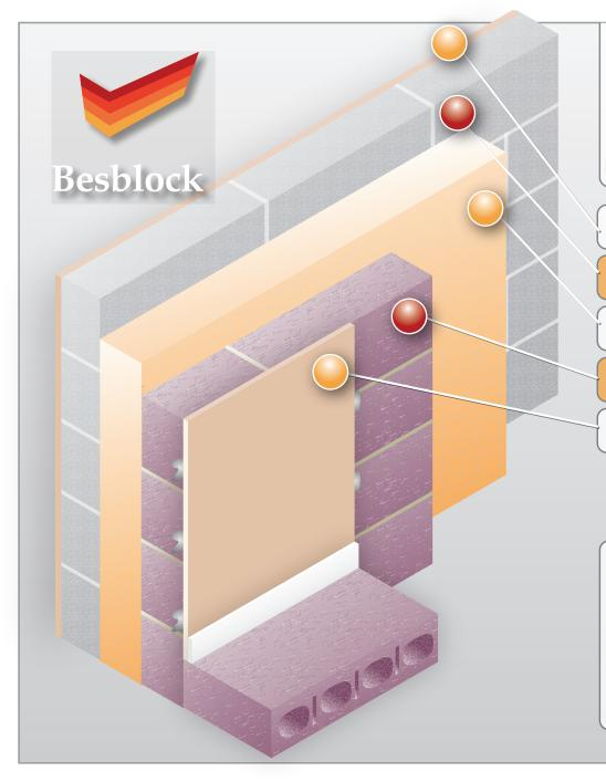
Star Performer Block Fully Filled Injected Cavity Wall
